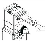
The inside of each switch features a device which holds the actuator in its closed position. Ideal for all those applications where several doors are unlocked simultaneously, but only one is actually opened. The device keeps all the unlocked doors in their position with a retaining force of 30 N~, stopping any vibrations or gusts of wind from opening them.
