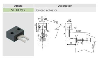
The actuator can flex in four directions for applications where the door alignment is not precise.
