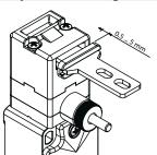
The actuation head of this switch features a wide range of travel. In this way the guard can oscillate along the direction of insertion (4.5 mm) without causing unwanted machine shutdowns. This wide range of travel is available in all actuators in order to ensure maximum device reliability.
